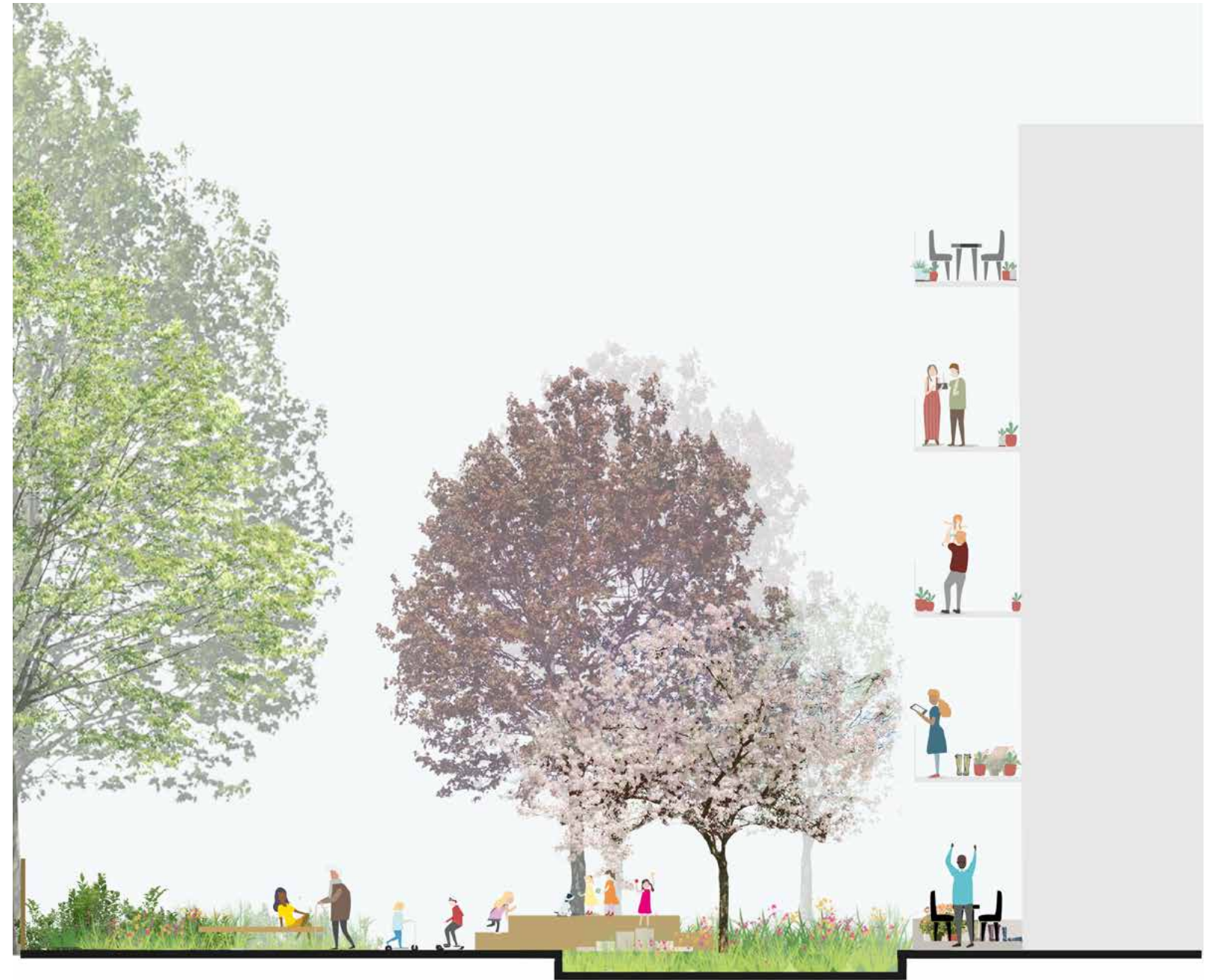
Vegetated edge with biodiverse hedges (3-5m) Paved route with play on the way elements and seating (3-10m) Rain garden (4-8.5m) Private Amenity (1.5m)
